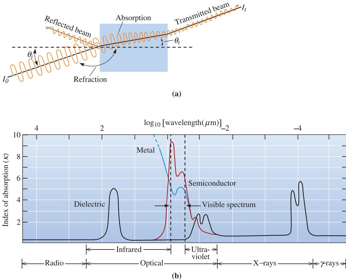
**Figure 21-2** (a) Interaction of photons with a material. In addition to reflection, absorption, and transmission, the beam changes direction, or is refracted. The change in direction is given by the index of refraction  $n$ . (b) The absorption index ( $\kappa$ ) as a function of wavelength.
