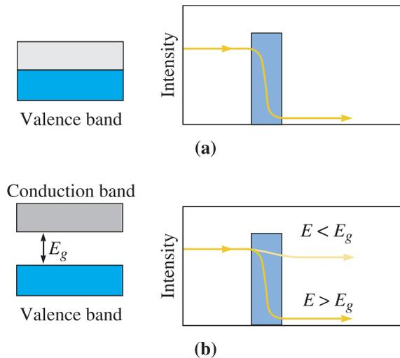
**Figure 21-6** Relationships between absorption and the energy gap: (a) metals and (b) dielectrics and intrinsic semiconductors. The diagram on the left represents the band structure of the material under consideration. The diagram on the right represents the intensity of light as it passes from air into the material and back into air.
