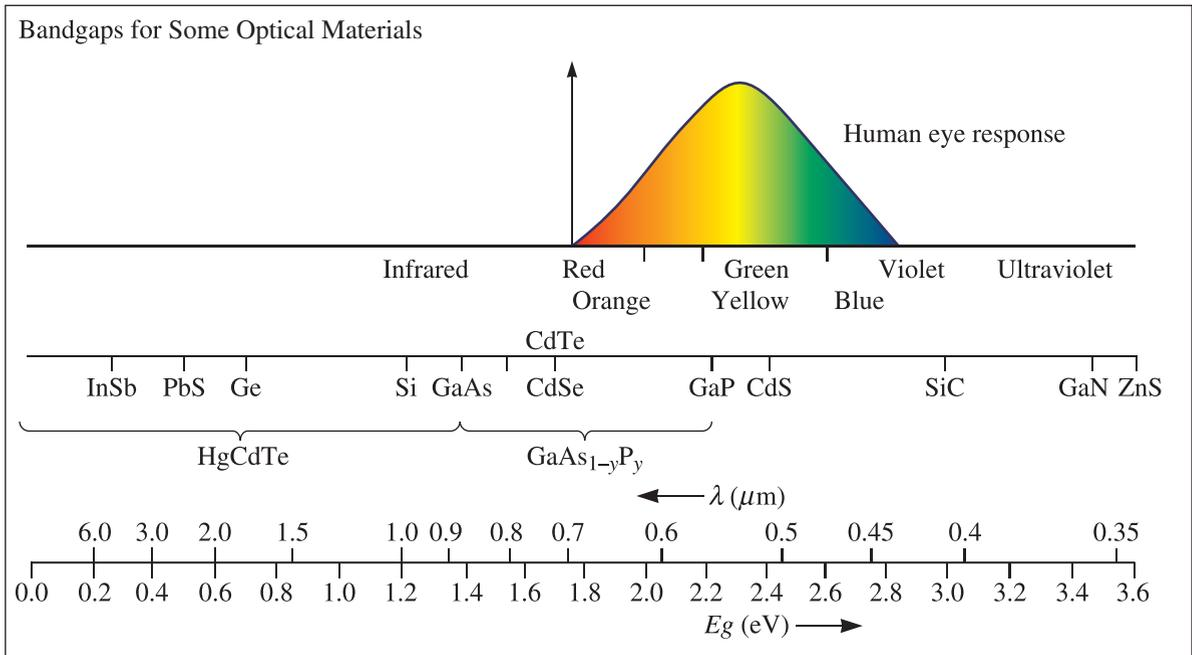
**Figure 21-1** The electromagnetic spectrum of radiation; the bandgaps and cutoff frequencies for some optical materials are also shown. (From *Optoelectronics: An Introduction to Materials and Devices*, by J. Singh. Copyright © 1996 The McGraw-Hill Companies. Reprinted by permission of The McGraw-Hill Companies.)
