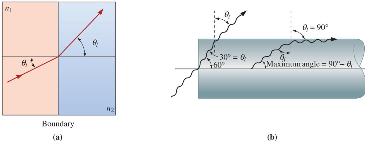
**Figure 21-3** (a) When a ray of light enters from Material 1 into Material 2, if the refractive index of Material 1 ( $n_1$ ) is greater than that of Material 2 ( $n_2$ ), the ray bends away from the normal and toward the boundary surface. (b) Diagram of a light beam in a glass fiber for Example 21-1.
