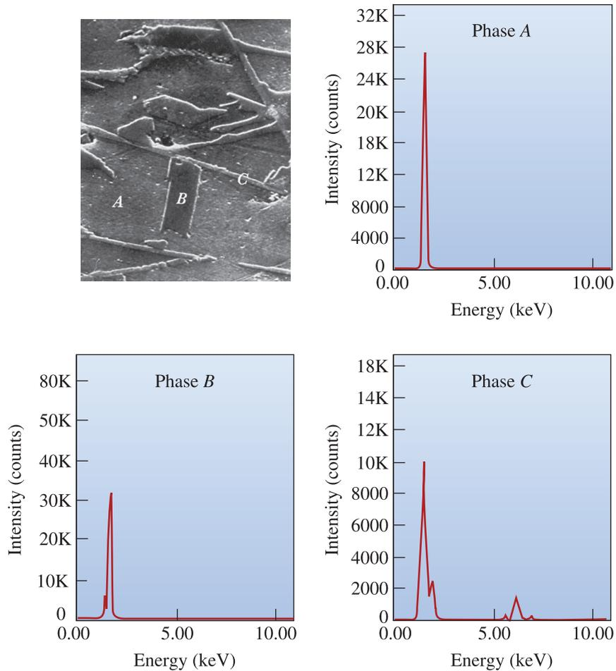
**Figure 21-13** Scanning electron micrograph of a multiple phase material. The energy distributions of emitted radiation from the three phases marked *A*, *B*, and *C* are shown. The identity of each phase is determined in Example 21-8. (Reprinted courtesy of Don Askeland.)
