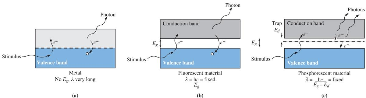
**Figure 21-14** Luminescence occurs when photons have a wavelength in the visible spectrum. (a) In metals, there is no energy gap, so luminescence does not occur. (b) Fluorescence may occur if there is an energy gap. (c) Phosphorescence occurs when the photons are emitted over a period of time due to donor traps in the energy gap.
