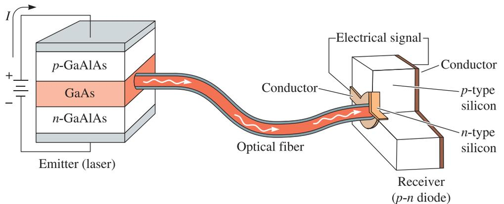
**Figure 21-8** Elements of a photonic system for transmitting information involves a laser or LED to generate photons from an electrical signal, optical fibers to transmit the beam of photons efficiently, and an LED receiver to convert the photons back into an electrical signal.
