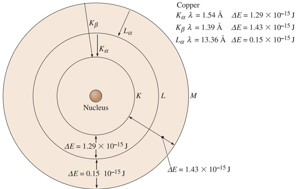
**Figure 21-11** Characteristic x-rays are produced when electrons transition from one energy level to a lower energy level, as illustrated here for copper. The energy and wavelength of the x-rays are fixed by the energy differences between the energy levels.
